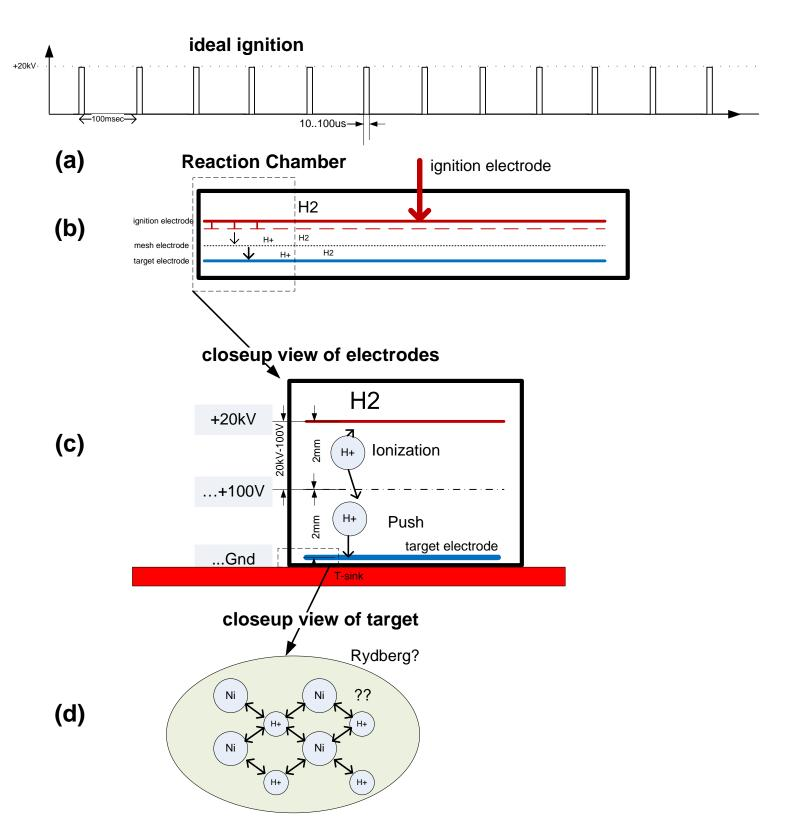
Note: 'ideal ignition' is not achievable. 'Real ignition' is bipolar without spwending considerable effort, and as such reduces the directivity of ion movement by say 50%. Typical ignition energy is 25..250mJ/ spark, which results in 5..50 J/second. i.e. 5..50Watt, which is a decent value. As such, the COP-limiting factor is probably not the energy of the sparking, i.e. the H+ generation, but the tbd thermal input, needed to start the reaction in the first place.
