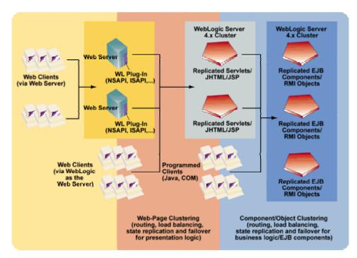
Three configurations of clustered BEA WebLogic Servers are supported. All three configurations use the same basic structure: a series of BEA WebLogic Servers all accessible over the same LAN, and accessible to a set of clients — browser servlet clients and Java application clients — over one of BEA WebLogic's various protocols. The three configurations supported are:
